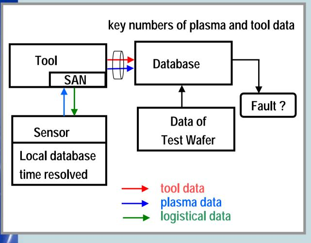
SAN integrated in the tool unification of data streams in the tool only key numbers of relevant data are stored
