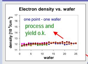
**Electron density** detects yield relevant process problem of CT etch pre- process in real time.
