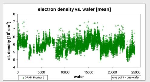
Mean value of electron density indicates chamber drift between wetcleans.
