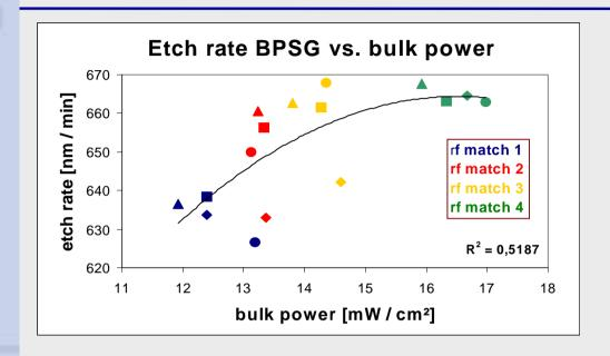
Task: Comparison of RF matchbox efficiency by measurement of bulk power dissipation inside the chamber (nominal RF generator power output is kept constant)
