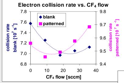
□ Variation of CF<sub>4</sub> flow in a CF<sub>4</sub> / CHF<sub>3</sub> / Ar gas mixture shows strong nonlinear impacts on electron collision rate and electron density
