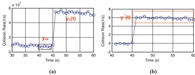
**Fig. 4.** Signals of collision rate for the step change test of source power: (a) raw signal of collision rate where  $y_{ss}$  is the average of steady state data points before step change and  $y_+(t)$  is the data point at the time before and after step change and (b) normalized signal,  $y^*$ .
