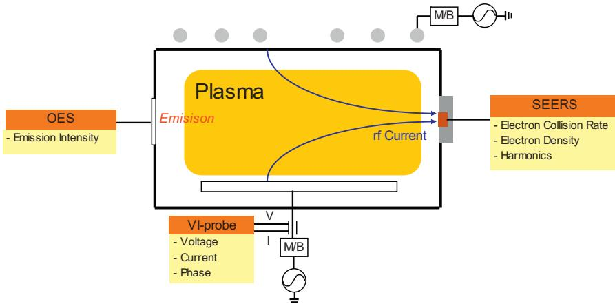
**Fig. 2.** Schematic of the plasma etching system and additional in situ sensors employed in this paper.
