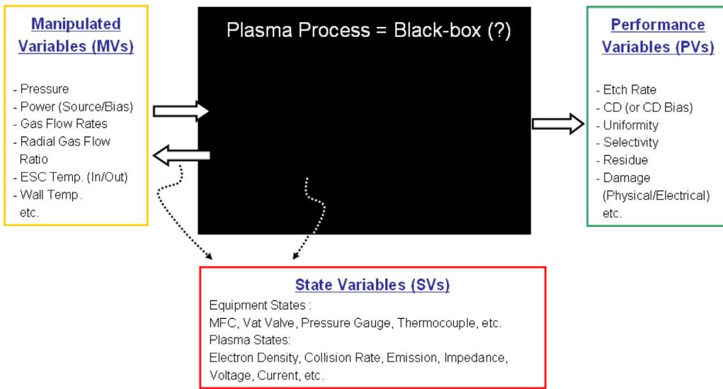
**Fig. 1.** Overview of complex multivariable plasma etch processes whose variables are classified into manipulated variables, state variables, and performance variables.
