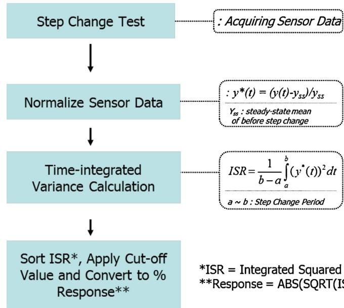
**Fig. 5.** A procedure for constructing a reference sensor library through ISR based sensor selection method.
