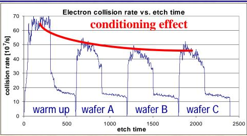
Electron collision rate shows conditioning impact and first wafer effect in real time
