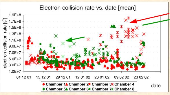
Drift of chambers 4 and 8 (mainly due to maintenance measures) was only detected by plasma parameter measurements
