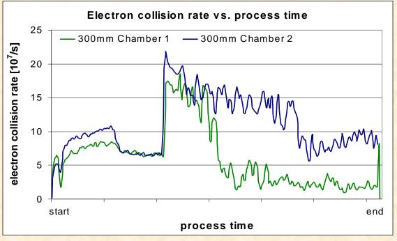
Nominal identical hardware and process in both chambers
