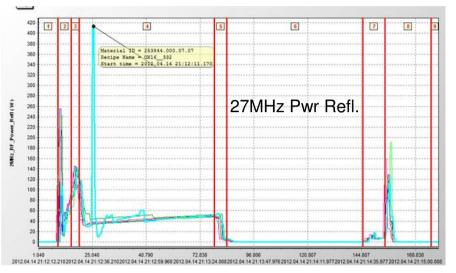
Plasma instabilities sometimes result in plasma dropout, sometimes it's recovering like in this case...but plasma parameters like collision rate show a remaining medium-term plasma instability and the product often is damaged without any tool alarm.
